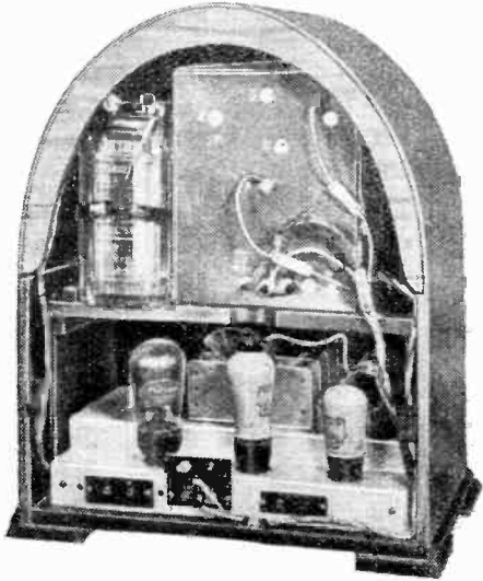
The Marconiphone Model 283 is typical of the inexpensive S.G. - detector - pentode battery receiver.
