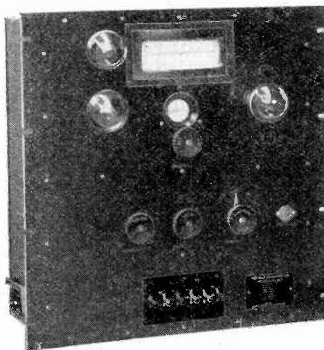
Fig. 6.—Measuring apparatus for routine maintenance tests on amplifiers and circuits.
