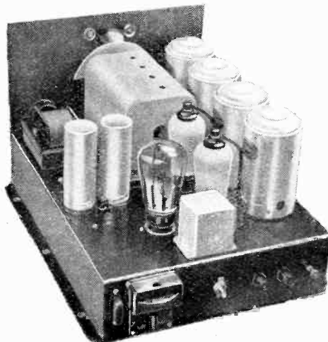
B.S.R. radio chassis for connecting to any L.F. amplifier.
